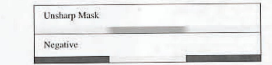
Fig.3: The registered sandwich is placed into the negative carrier and printed together with the emulsion side down. The increase in required paper contrast and the "edge effect" create a sharper image.
