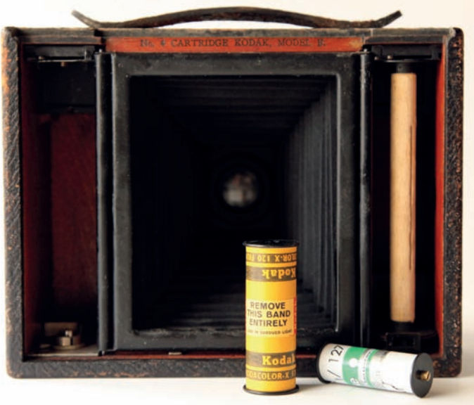
Kodak no. 4 camera, taking the mighty 5" wide '123' format (discontinued 1949) and yielding 5 x 4" images. Contrasted with normal 120 and 127 films.
