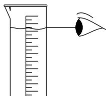
**Accurate Measurement** is essential. Always read the liquid level at the bottom of the meniscus.
