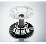
Fits all tanks (except 2513) in the 2500 system. The reel can be adjusted for various film sizes and film can be loaded with or without loader. The reel is designed for professional use and holds up to six sheet films of size 6x9 / 9x12 / 4x5''.
